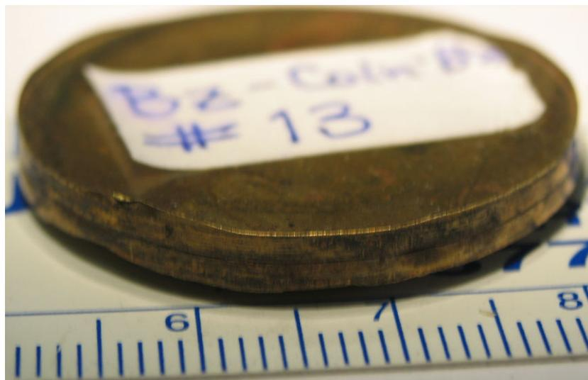
**Figure 17.** General view of brass-nickel-alloy coin-brass plates welded by the water projectile impact in at the water velocity 750 m/sec (Table 1, Exp. #13).
