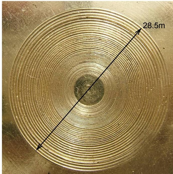
**Figure 6.** General view of concentric grooves and ridges formed on the surface of brass sample. Notice precise geometry of the generated grooves.
