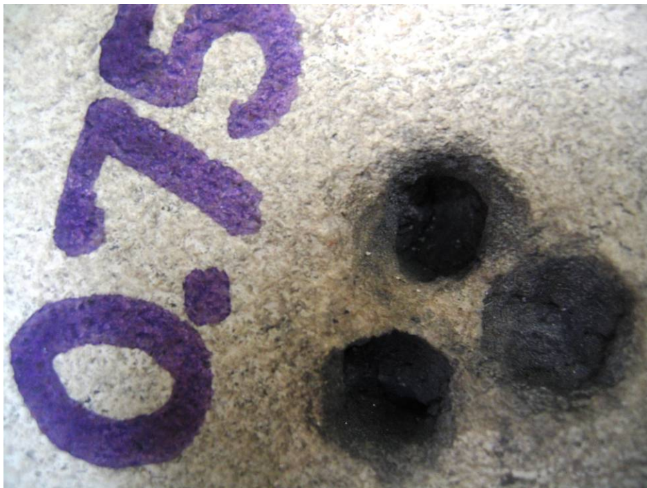
Figure 15. Three impacts at the distance of \frac{3}{4} " between axes of impact zones. Notice minimal interference.
