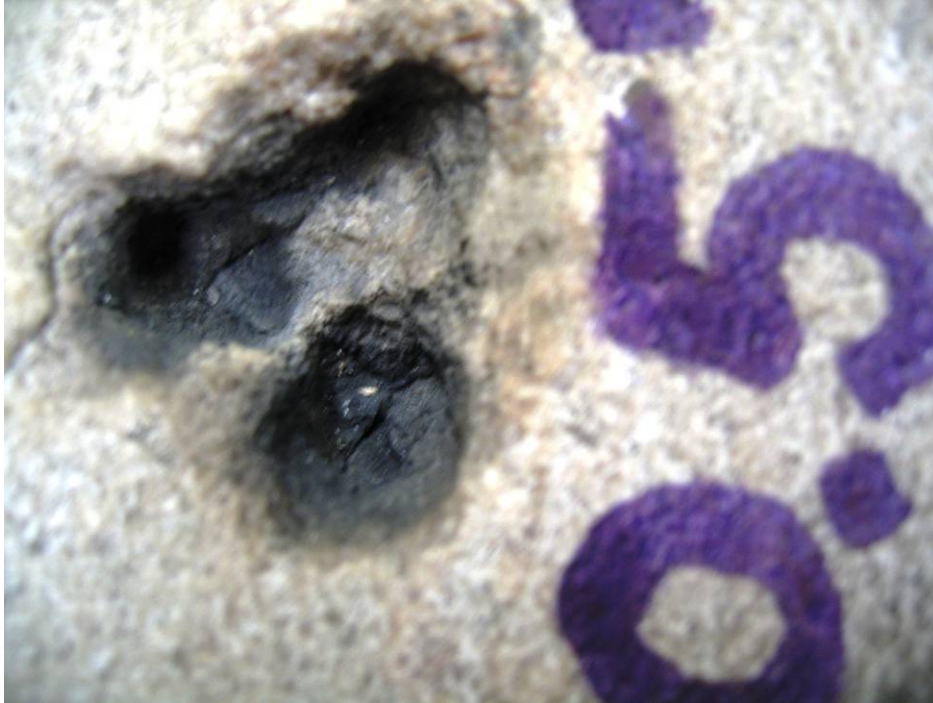
Figure 16. Three impacts at the distance of \frac{1}{2} " between axes of impact zones. Notice significant interference between two shots.
