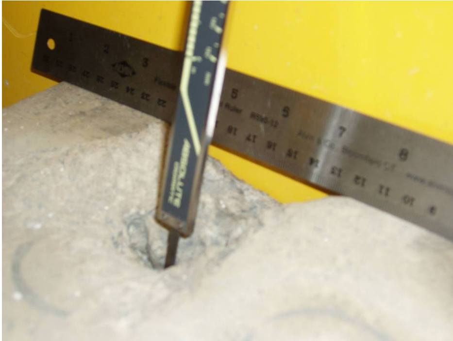
Figure 12. Boring of a granite by 52 sequential impacts. Notice dimensions of the generated cavity.
