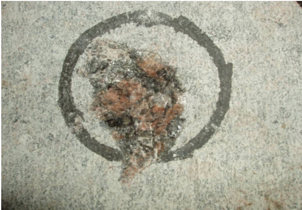
Figure 19. Granite removal by impact of a projectile generated by low-power launcher.
