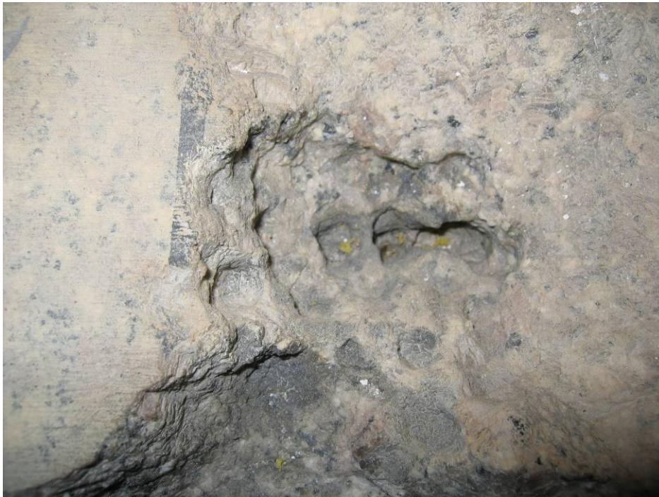
Figure 13. Boring of a granite by 52 sequential impacts.
