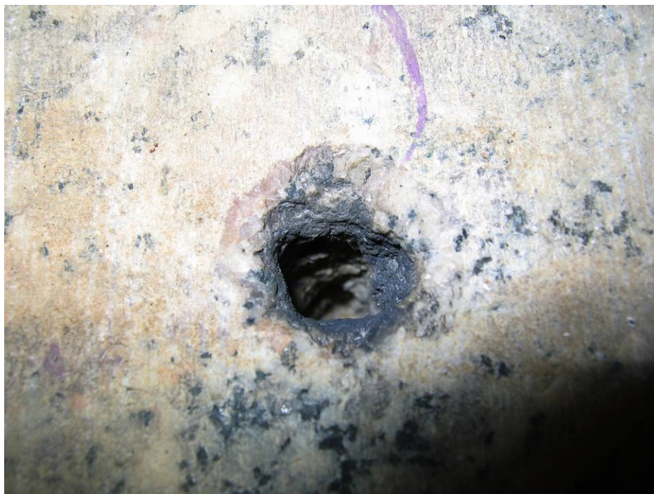
Figure 11. Boring of a granite plate by sequential impacts of projectiles at the same site.
