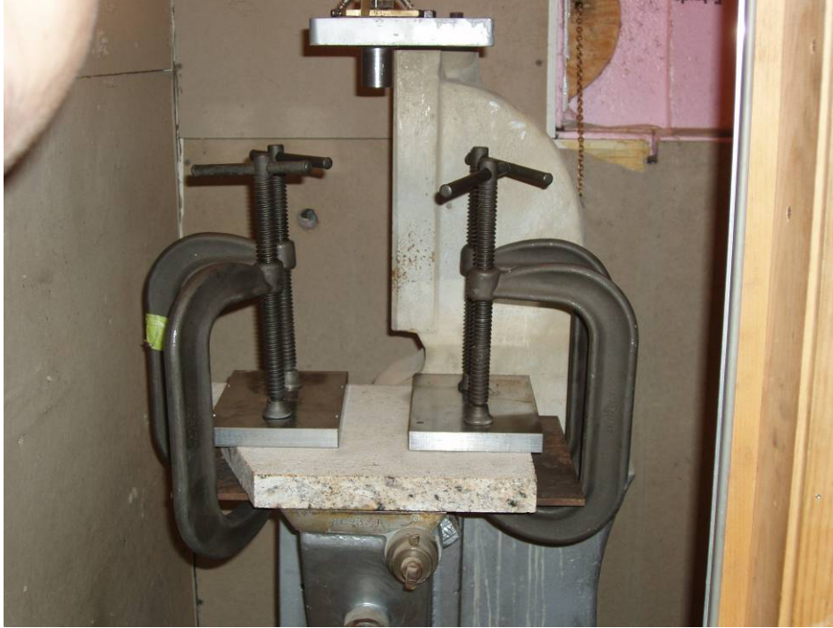
Figure 18. Setup for granite boring at induced compressive stresses.
