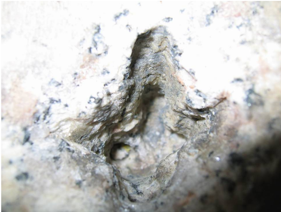
Figure 17. Boring of a granite plate by sequential impact with a cross-like pattern of impact distribution.
