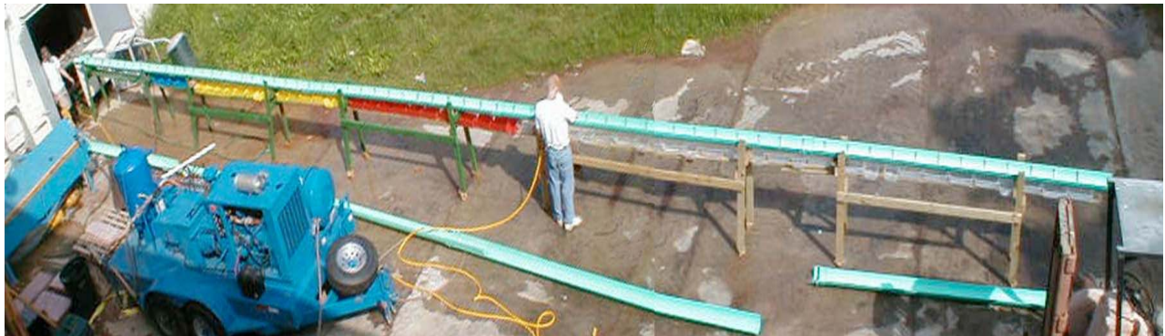
Figure 1: Tube tests for measurement of energy of ASJ.
