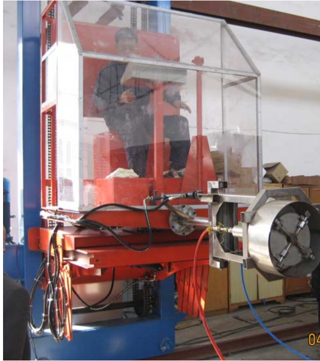
Figure 6. Locomotives Rust Removal Equipment
