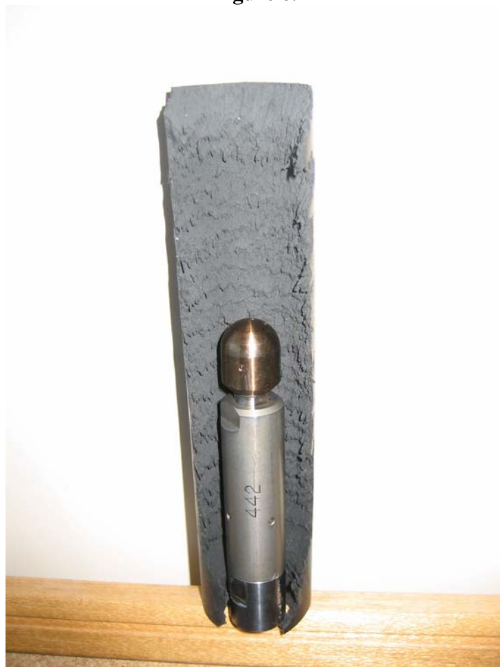
Material Not Removed by Nozzle C in a 35 mm Tube Figure 7.
