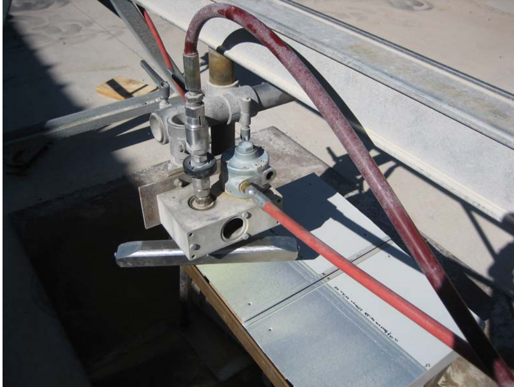
Test Arrangement Consisting of a Rotating Head and Traversing Mechanism Figure 1.
