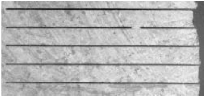
Figure 6 Entrance of waterjet in the granite
