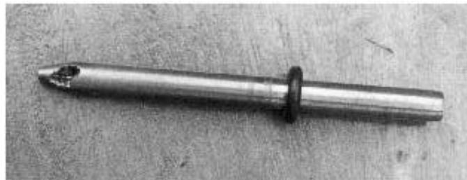
Figure 8 Mixture tube nozzle destroyed by synthetic abrasive.
