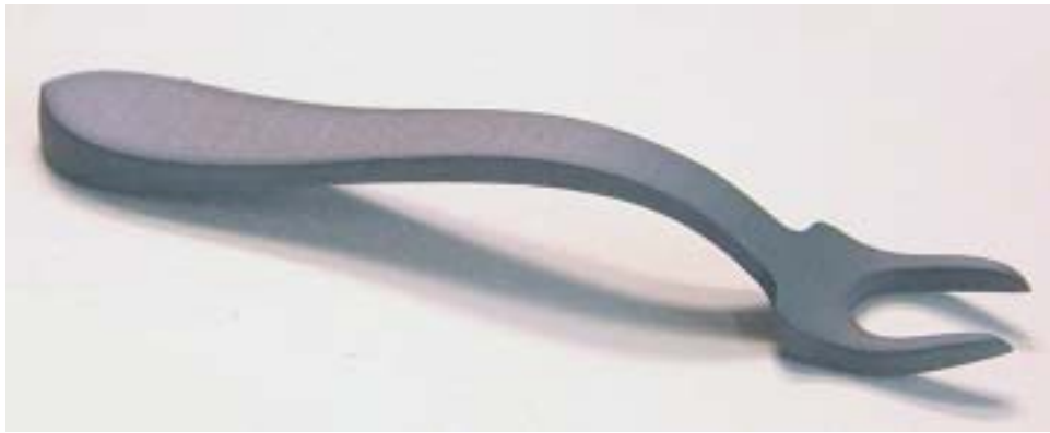
Figure 2. A complex part machined indexing the b-axis between two consecutive cutting cycles.
