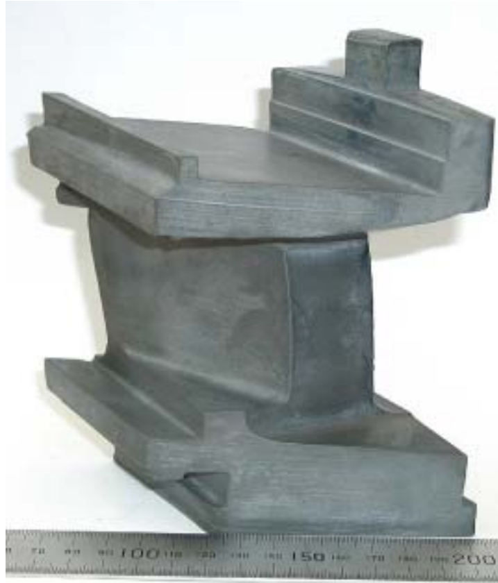
Figure 7. Finished rough machining of the guide vane using 4-axis AWJ cutting.
