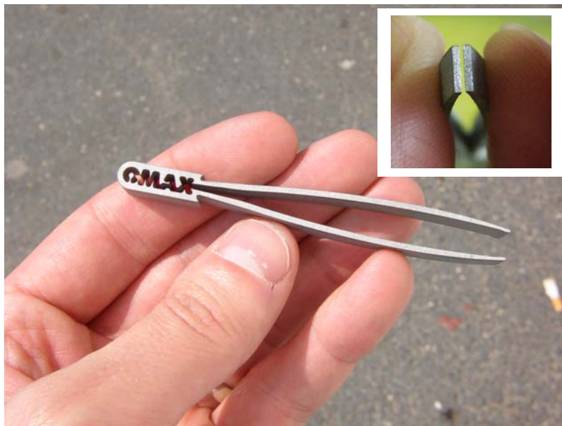
Figure 20. A pair of tweezers cut with a tilting head showing taper-free tips
