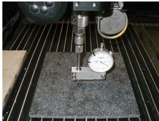
Figure 14. Squareness calibration tool in action
