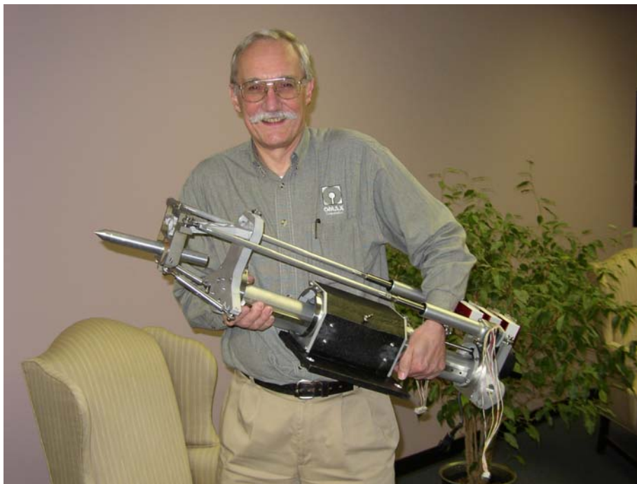
Figure 4. Initial design of tilting head with two linear actuators
