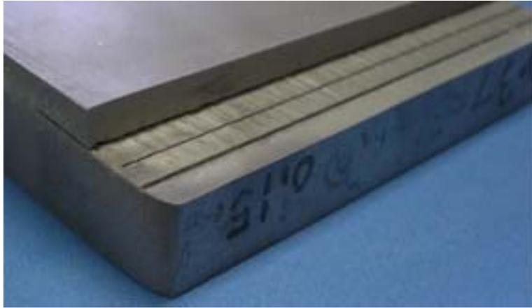
**Figure 11.** Precision depth cutting to isolate blocks of material.
