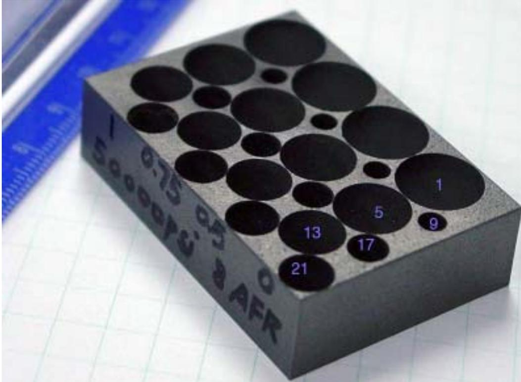
**Figure 7.** Initial pattern of test holes, the numbers shows the order in which each series of four holes at the same size, but differing nozzle angle, are cut.
