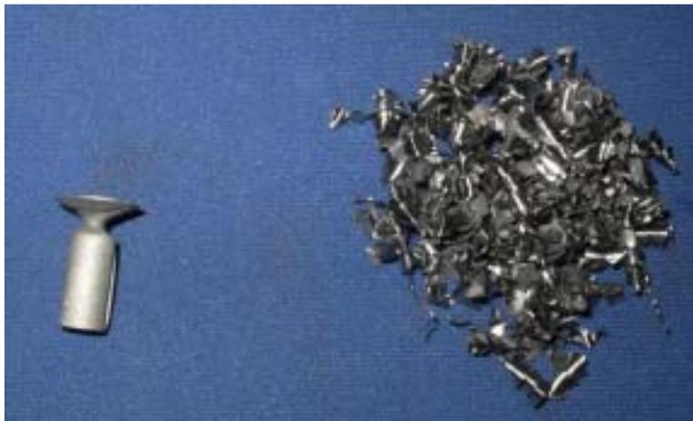
**Figure 10.** AWJ cut chamfered hole scrap contrasted with conventional machining scrap.
