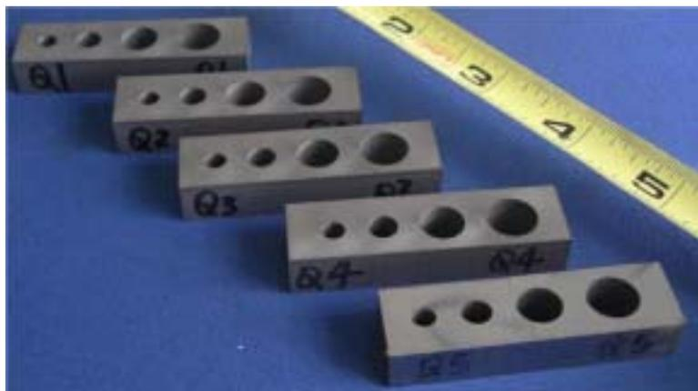
**Figure 2.** Initial holes cut in titanium at different cut qualities.
