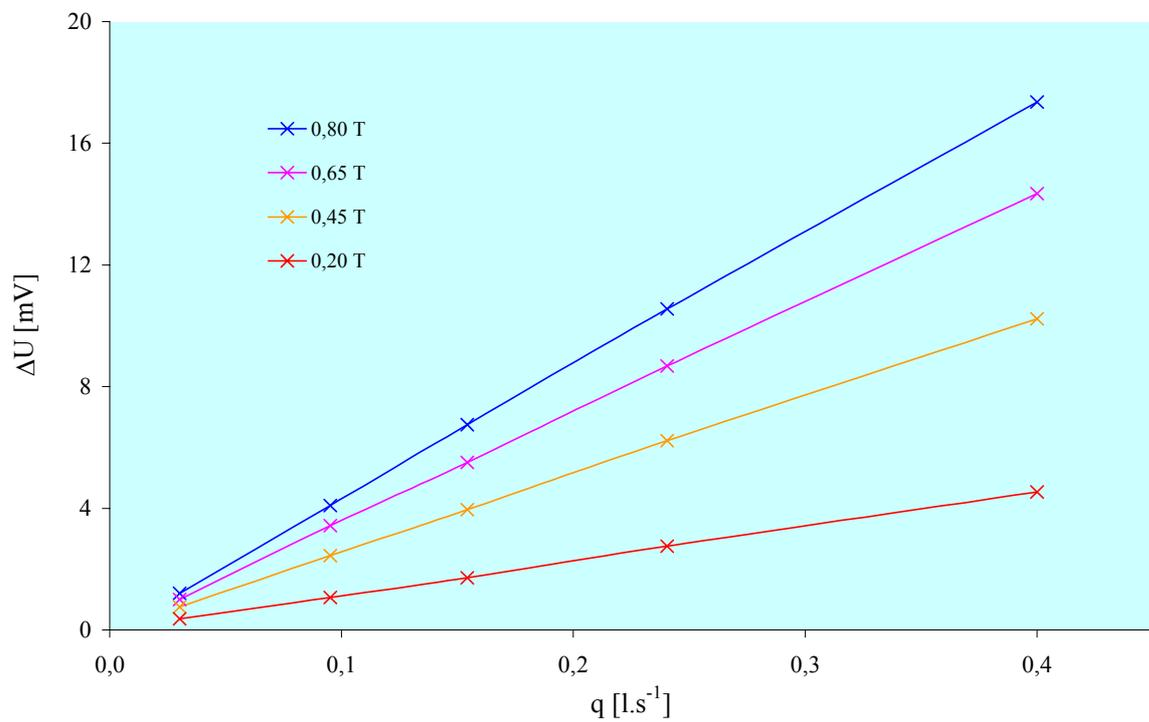
**Fig. 2.** The growth of the voltage change  $\Delta U$  on the side electrodes with growing flow rate  $q$ .
