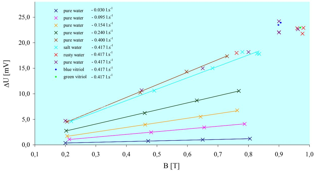
**Fig. 3.** The growth of the voltage on the electrodes  $\Delta U$  with growing magnetic field induction  $B$ .
