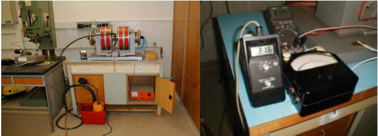
**Fig. 1.** Measurement of the magnetohydrodynamic effects in liquids: left side - the configuration; right side - the detail of measuring apparatus.
