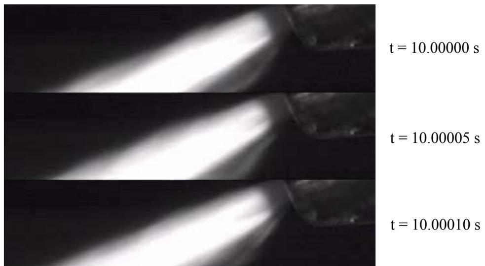
**Figure 4** Series of stills taken from the high-speed video imaging of the jet running at 6000 psi (41.1 MPa); the interval between images is  $5 \times 10^{-5}$  s.
