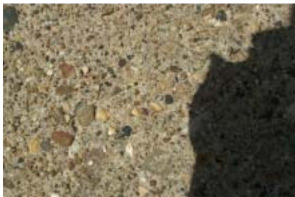
TEST ZONE #2 SpinJet with Vacuum Recovery – Clean Surface, no dust, No dirt, no moisture, of and kind.
