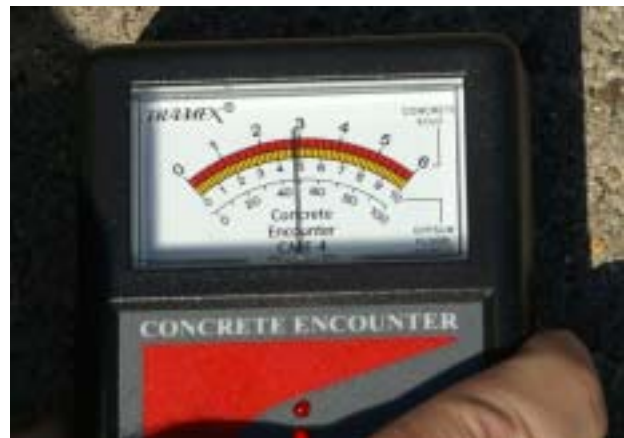
Test Zone #2 SpinJet with Vacuum Recovery – Moisture Reading at two minutes after jetting: 2.9% H2O.
