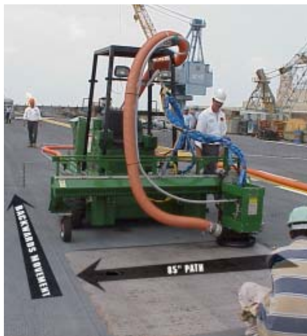
Figure 6. Second generation systems not only traverse backwards, but can index the nozzle array from side to side allowing for up to an 85" cleaning path.
