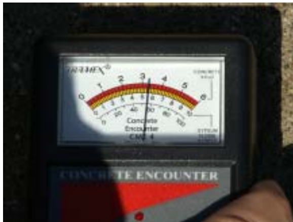
TEST ZONE #2 SpinJet with Vacuum Recovery – Moisture Reading at one Minute after jetting: 3.3% H2O.
