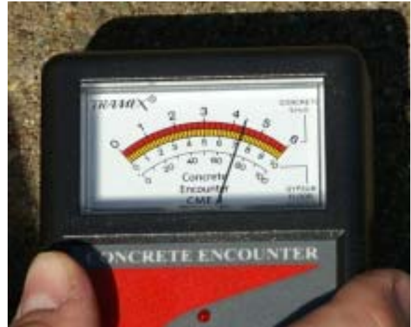
TEST ZONE #2 SpinJet with Vacuum Recovery –Moisture Reading at five seconds after jetting: 4.4% H2O.
