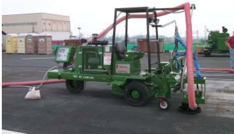
Figure 5. Second generation coating removal systems combine the advantages of the original systems with new features that improve productivity.
