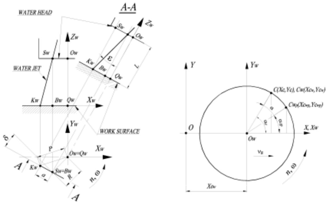
**Figure 7.** Analytical schema of surface treatment using one-orifice rotary nozzle
