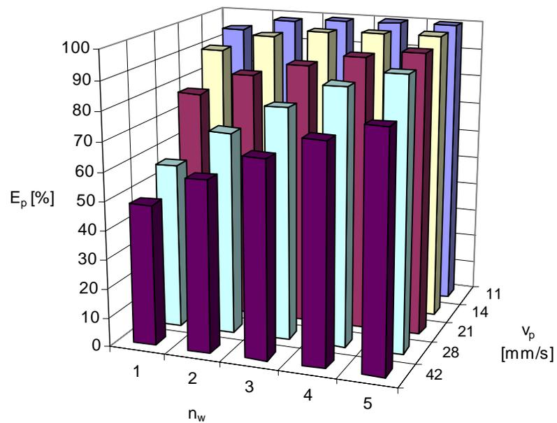
**Figure. 11.** Influence of water orifices number and rotary nozzle feed rate on flat surface treatment effectiveness for  $n=1,7$  s<sup>-1</sup>,  $d_w=0,4$  mm,  $L=100$  mm
