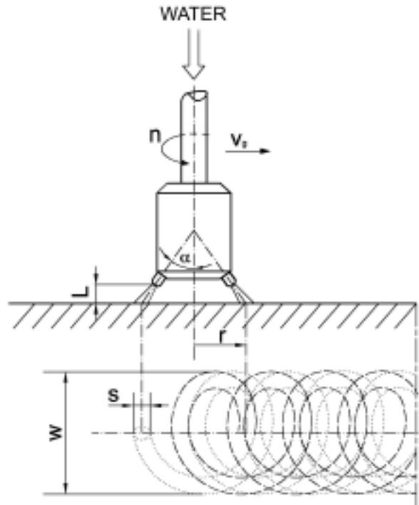
**Figure 1.** Schematic view of flat surface treatment using rotary head equipped with two water nozzles
