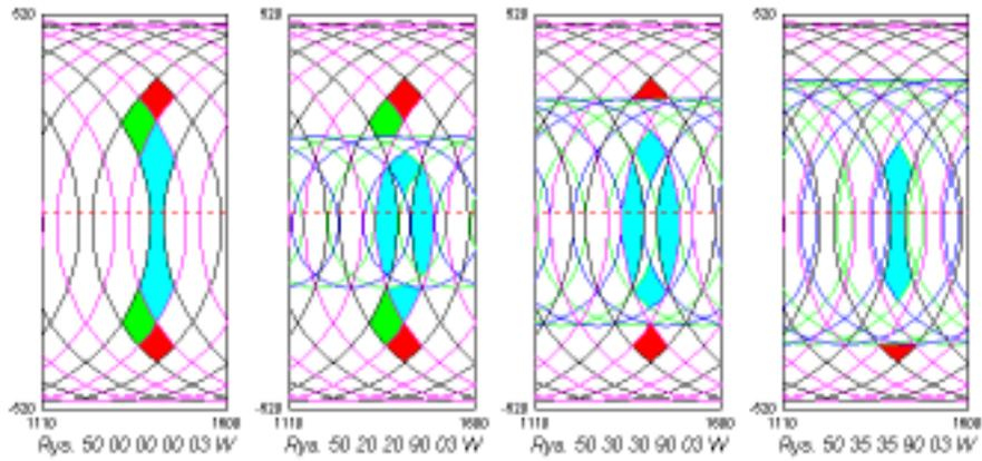
**Figure 5.** Influence of two extra orifices characterized by different radius displaced in  $90^\circ$  regarding 1 and 2 orifices on post-machining marks concentration.
