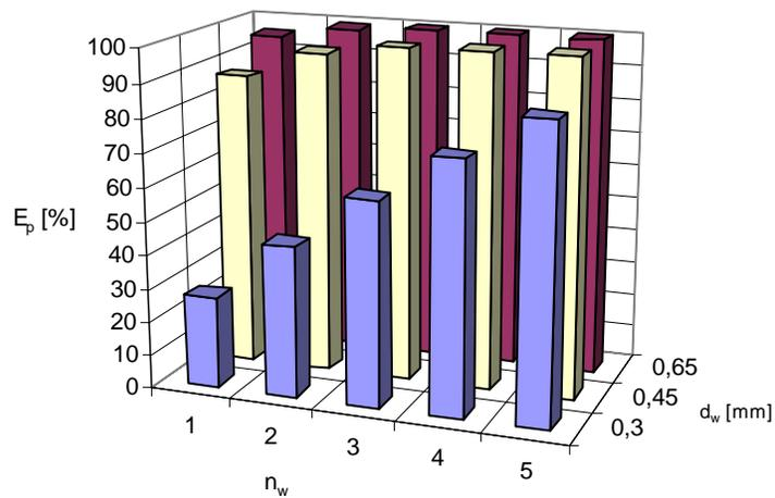
**Figure. 9.** Influence of water orifices number and their diameter on flat surface treatment effectiveness for  $n=1,5 \text{ s}^{-1}$ ,  $v_g=25 \text{ mm/s}$ ,  $L=100 \text{ mm}$
