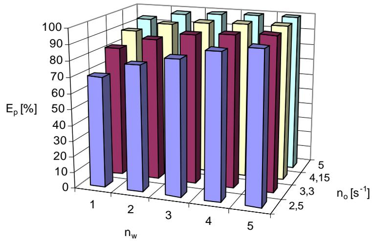
**Figure. 10.** Influence of water orifices number and nozzle rotary velocity on flat surface treatment effectiveness for  $d_w=0,35$  mm,  $v_g=26$  mm/s,  $L=100$  mm
