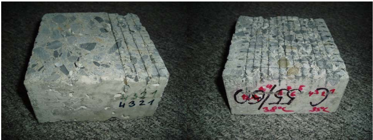
Fig. 9. Sample of concrete: blue (green) marked kerfs 1 through 4 are cut in air at four different traverse rates. Red kerfs are cut in water: 1 through 4 in pressure 1.2 MPa, 5 through 8 in pressure 0.6 MPa and 9 through 12 in 0.1 MPa (without any additional pressure, just near the water level). Four traverse rates were used with each pressure inside the pressure vessel.
