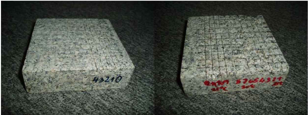
Fig. 8. Sample of granite: blue marked kerfs 0 through 4 are cut in air at five different traverse rates. Red kerfs are cut in water: 1 through 4 in pressure 1.2 MPa, 5 through 8 in pressure 0.6 MPa and 9 through 12 in 0.1 MPa (without any additional pressure, just near the water level). Four traverse rates were used with each pressure inside the pressure vessel.
