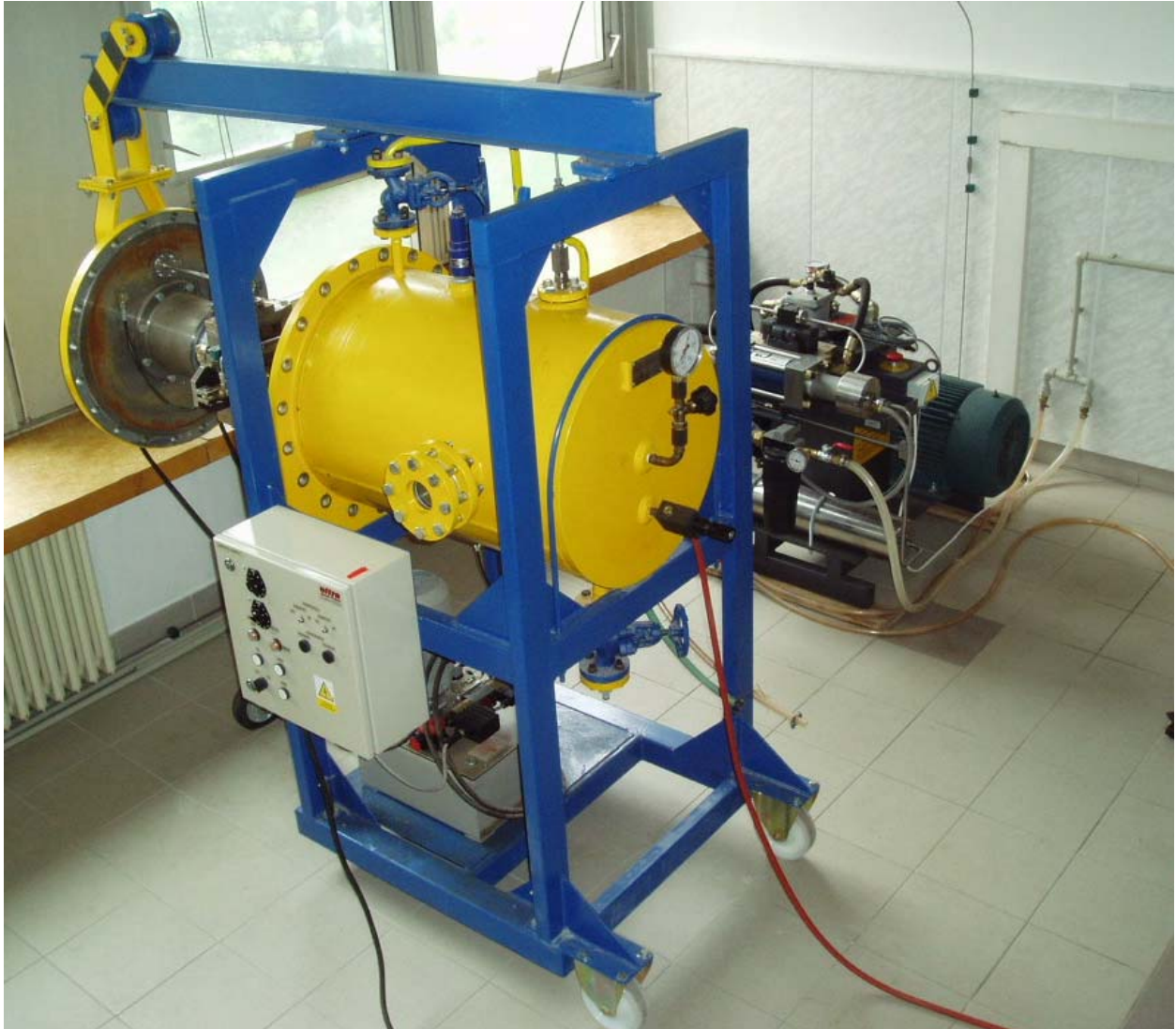
Fig. 1. View of the mobile pressure vessel, the high-pressure pump for water jet generation and vessel feeding and their location in our laboratory.
