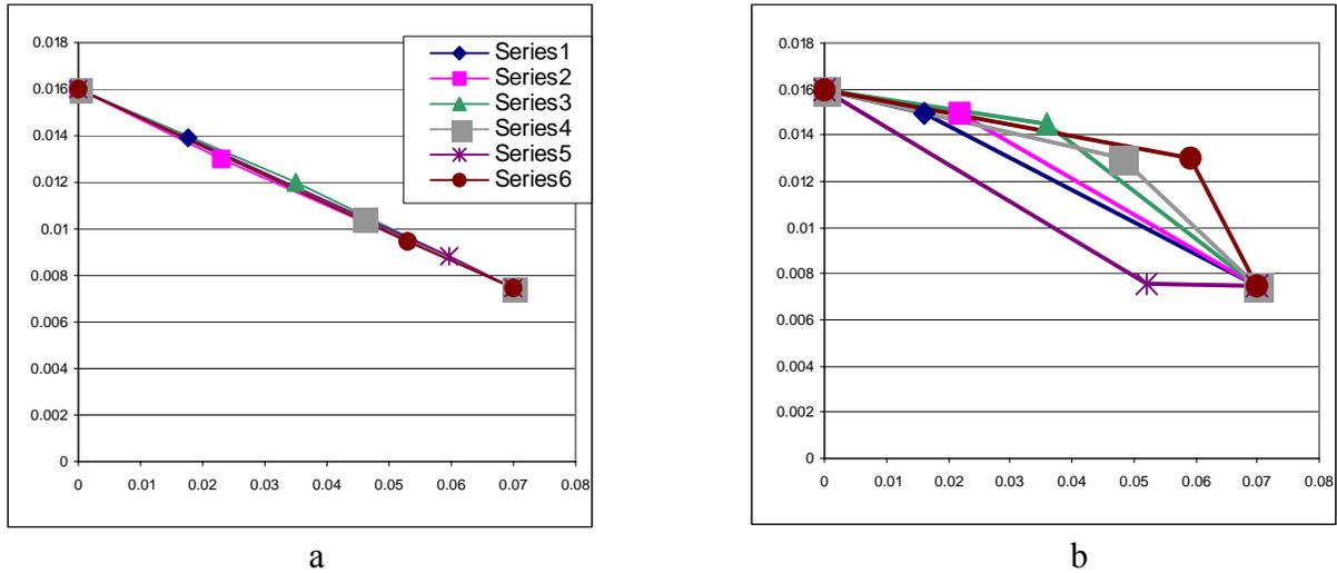
**Fig. 10 Initial a) and optimized b) nozzle profiles**
