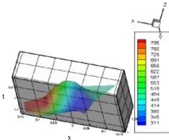
**Fig. 4 Water velocity distribution plot with 100g water load**
