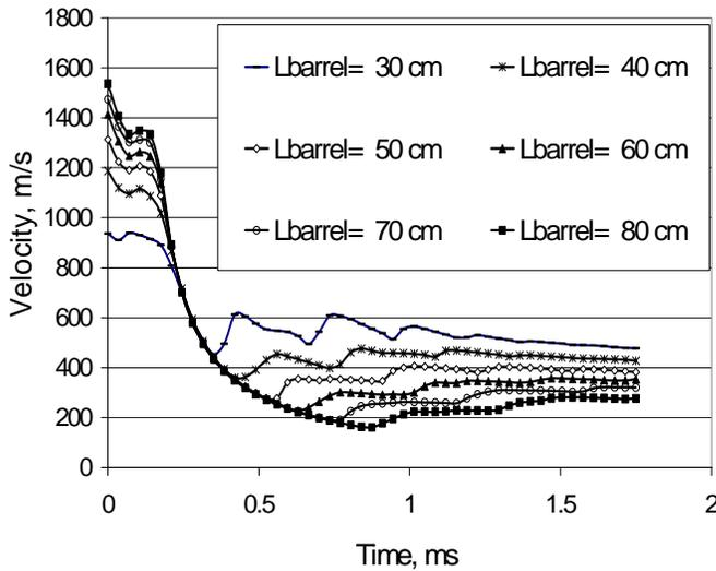
**Fig. 3 Outflow velocity vs. time at diff. barrel length**
