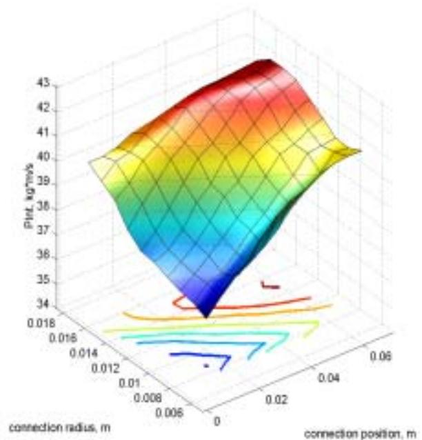
**Figure 11 Effective momentum integral of a slug at different nozzle configurations.**
