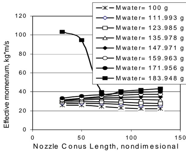
**Fig. 6 Impulse Integral vs. Water Load**
