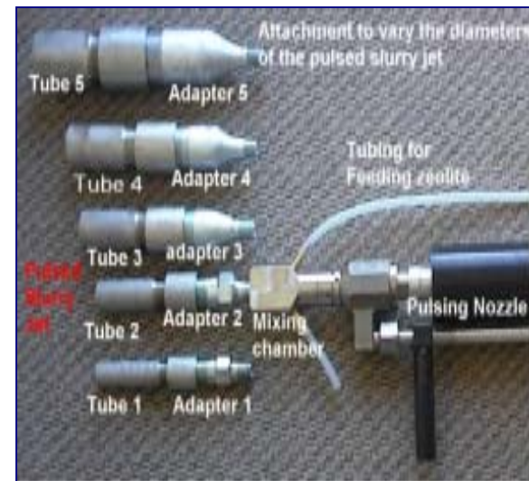
Fig. 4. A general view of the components fabricated for producing AFPJ.
