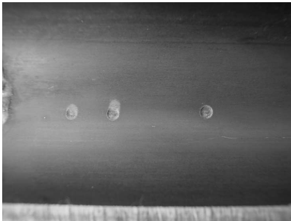
Damage to Carbon Steel Tubing, at 140 MPa (20,000 psi) with Stationary Drilled Steel Nozzle, for Time Periods of 10, 30 and 60 Seconds Figure 4.
