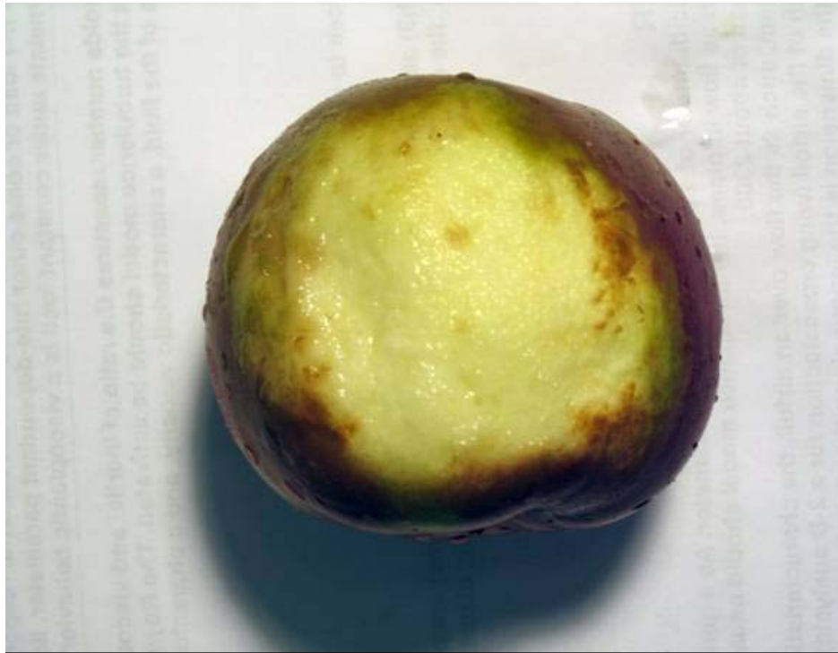
Figure 9 Apple after Ice Jet Peeling
