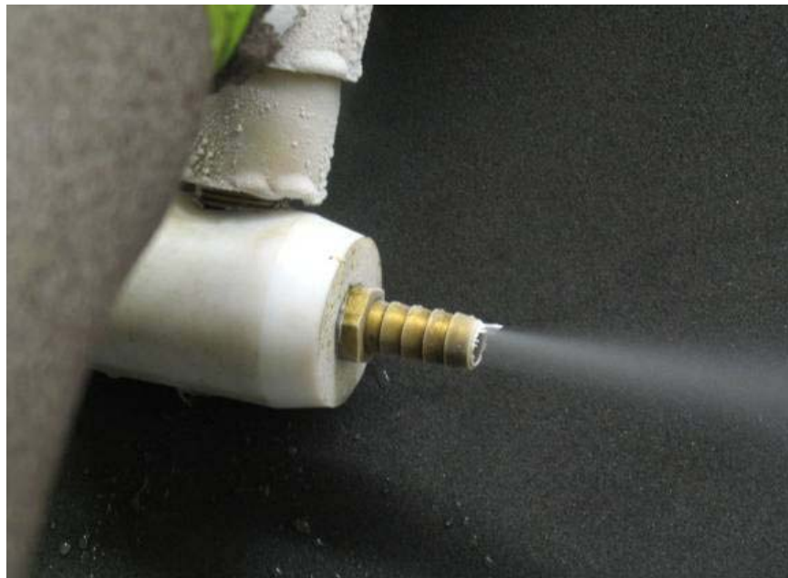
Figure 5 Nozzle with Visible High Speed Ice Jet
