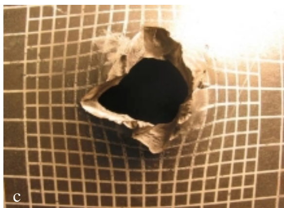
Figure 11. a) Two 9.9 mm thick Aluminum plates simultaneously pierced by 230g water-projectile with 57 g of rifle powder charge; b) Captured fragments; c) Top view of front plate; d) Top view of back plate.
