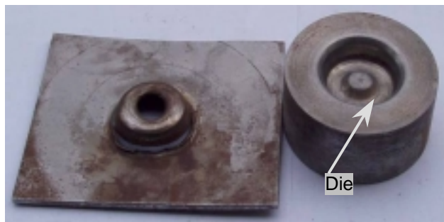
Figure 8. Formation of a 3D shape in the course of the liquid impact ( h=2.5 mm, D=25 mm, max. depth 10 mm). Notice the compliance of geometries of the die and the generated part.
