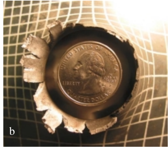
Figure 10. a) Side view of three 4.8 mm steel plates simultaneously pierced by 230g water projectile with 64.69g of rifle powder charge; b) Top view back plate.
