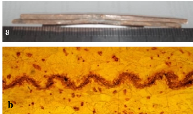
Figure 12. a) Copper plates joined by the water impact at the water velocity 1500 m/sec and h=3 mm. b) Micrograph of wavy interface of joined copper plates.
