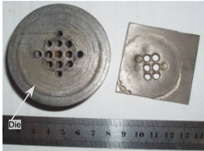
Figure 6. Formation of the multiple openings by a single impact of a round jet. Steel sheet thickness is 2.5 mm and the opening diameter is 4 mm. Notice that the liquid penetration into the workpiece can be controlled by the impact condition.
