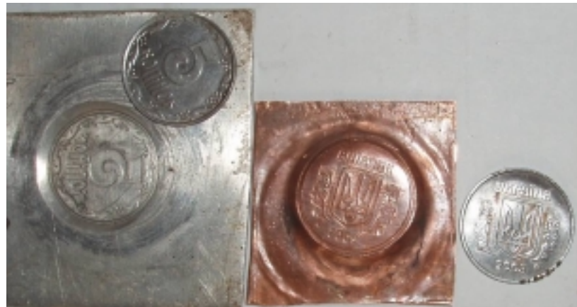
Figure 9. Printing of a coin (24 mm diameter and 1mm thick) against 2 mm aluminum alloy (left) and 1 mm copper (right) sheets. Notice precision reproduction of the die geometry.
