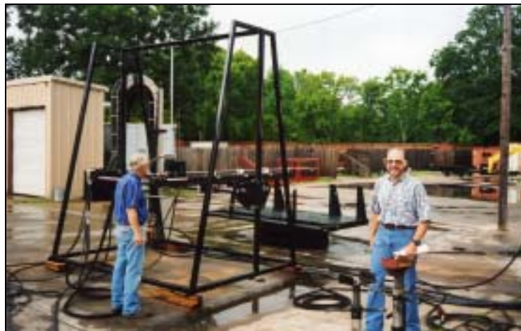
Figure 5 – Indexer Device for Chlorine Cell Cleaner
