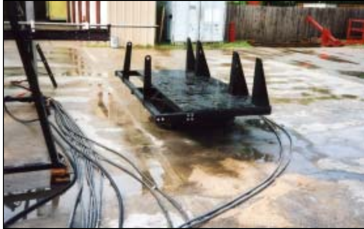
Figure 6 – Rotating Device for Chlorine Cells
