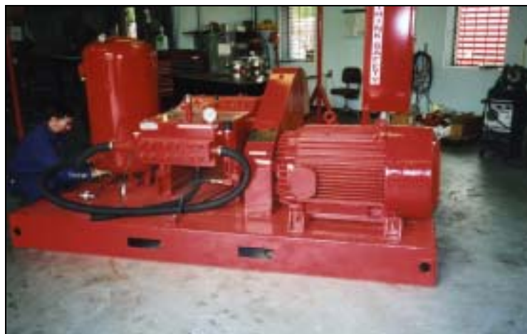
Figure 8 – 300 horsepower pump unit
