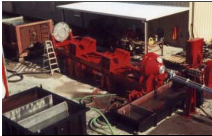
Figure 9 – Rocket Washout System
