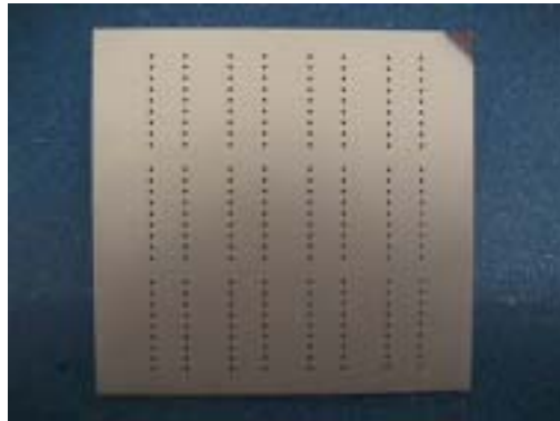
Figure 10: AWJ-Drilled Holes in ALN Material Substrate
