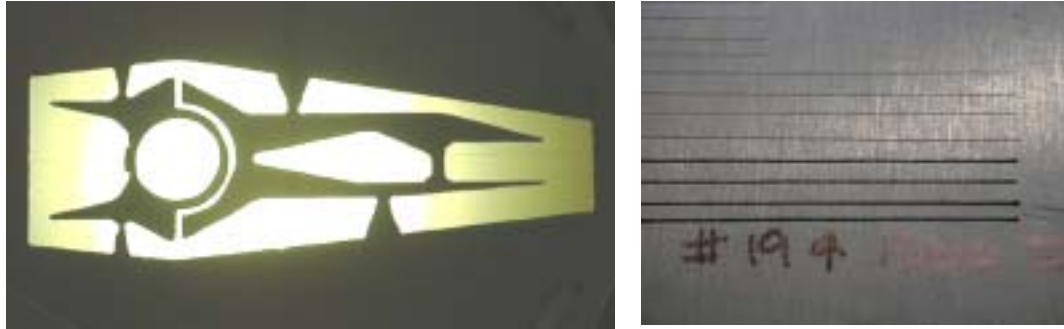
Figure 8: WJ-Cut in 20-mm long Micro Hard Disk Composite Arm
