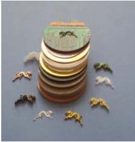
Figure 3 Sample materials cut with 50micron diameter jet – includes metals, polymers, glass and composites
