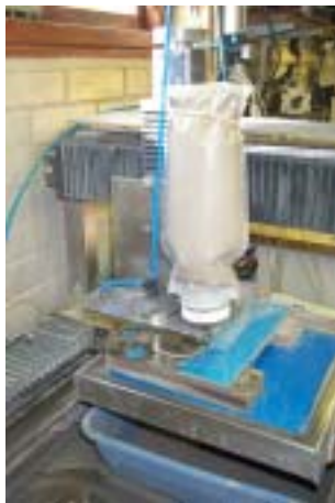
Figure 5 90micron diameter FAW cutting head fed from a transportation pouch
