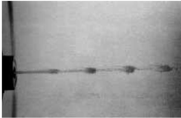
Figure 1. Example of Percussive Jets. A small cyclic variation or modulation impressed on a steady discharge of water causes the free jet to become bunched. Consequently the jet will strike a target in a sequence of sharp impacts rather than steadily.
