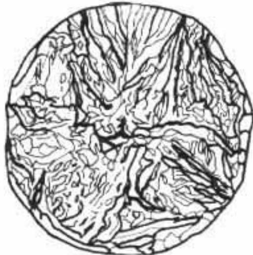
Figure 2. Entrained air bubble filled with chloride crystals.
