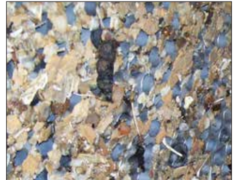
Macro Fouling Inhibiting Flow
