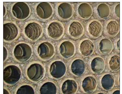
Scale Build-up on Tubes
