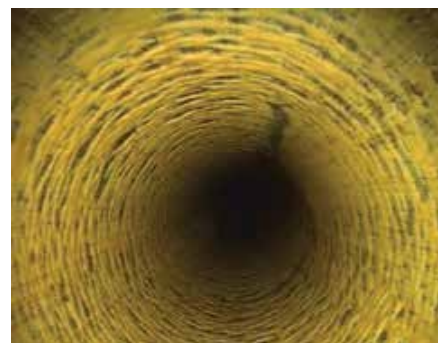
Stainless Steel Tube with Scale Deposits
