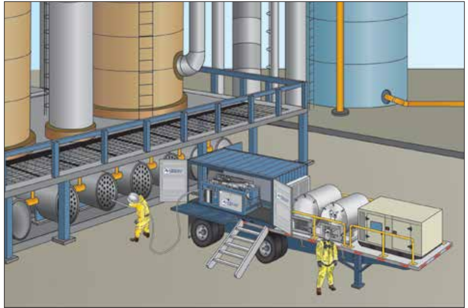
NitroLance Cleaning Heat Exchanger Tubes at Refinery
