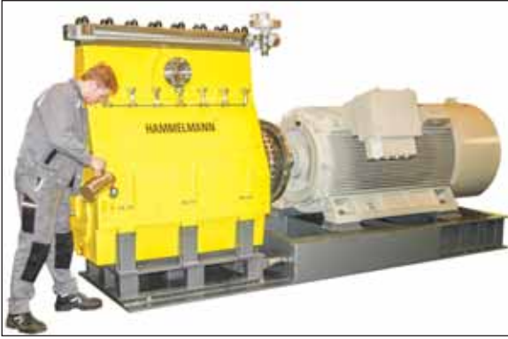
HDP-MC (1500 hp) pump manufactured for industrial cleaning and chemical injection.
