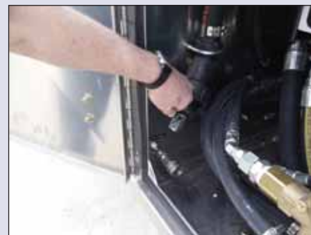
Hoses and fittings should be inspected on a daily basis.
