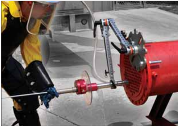
The APS-designed Articulated Flex Lance Safety Stop also known as the "Chicken Wing."
