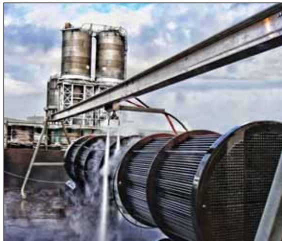
Bundle Blaster automated system for external cleaning of heat exchangers and tube bundles.
