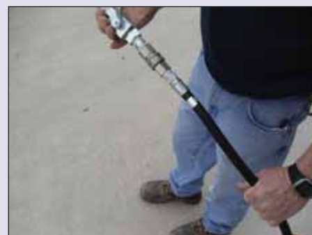
The handguns and water lances on a hydro excavator should be inspected to ensure they are in proper and safe working order.
