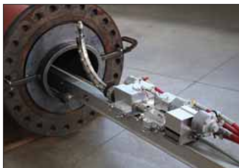
StoneAge Boiler Tube Cleaner safely cleans radial tubes found in mud drums of package boilers.
