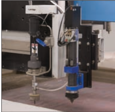
Pneumatic drills allow waterjet operators to pre-drill materials that are sensitive to delamination prior to waterjet cutting them. Courtesy Jet Edge, Inc.
