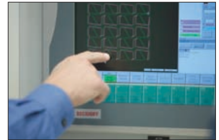
Nesting software maximizes the quantity of parts that can be cut out of a piece of material, reducing material waste and speeding production. It also can tab parts to prevent them from falling into the waterjet tank or keep them together on a plate for faster loading and unloading. Courtesy Jet Edge, Inc.
