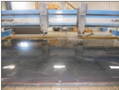
Precision Waterjet Concepts equipped their Jet Edge waterjet system with mirroring capabilities. This allows them to cut large parts twice as fast by cutting the part with two cutting heads. Photo courtesy Precision Waterjet Concepts
