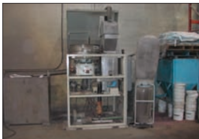
G.O. H2O of Edmonton, Alberta, Canada, is successfully recycling garnet abrasive by mixing the recycled abrasive with new abrasive. They have not noticed a reduction in cutting speed. Their abrasive recycling system paid for itself within one year. Courtesy G.O. H2O.
