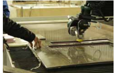
Neolith material being cut with Dynamic XD on a Flow Mach 3 waterjet.
