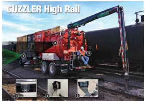
Mounted on the front and sides of the Guzzler High-Rail vacuum loader, the optional camera system provides a wide-area, real-time view of the surroundings while the unit is vacuuming on railroad tracks and in switchyards.
