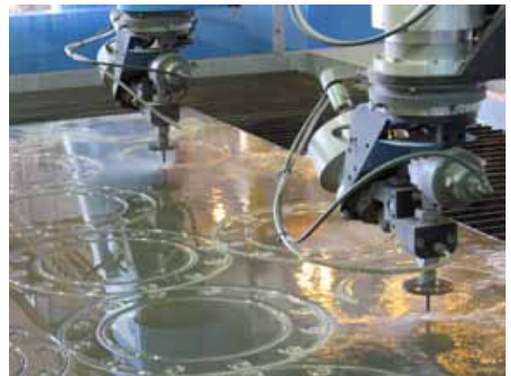
Jet Edge's EDGE X-5 5-axis waterjet cuts precise 3D parts from virtually any material.
