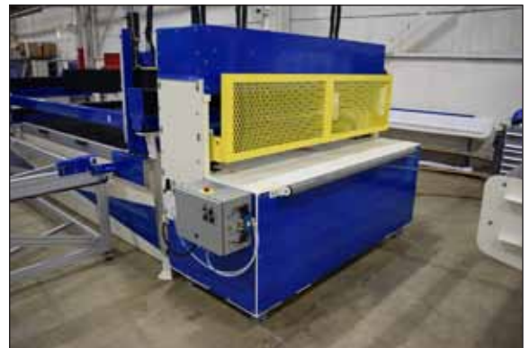
The pinch feed roller helps to guide the material evenly into the cutting area.
