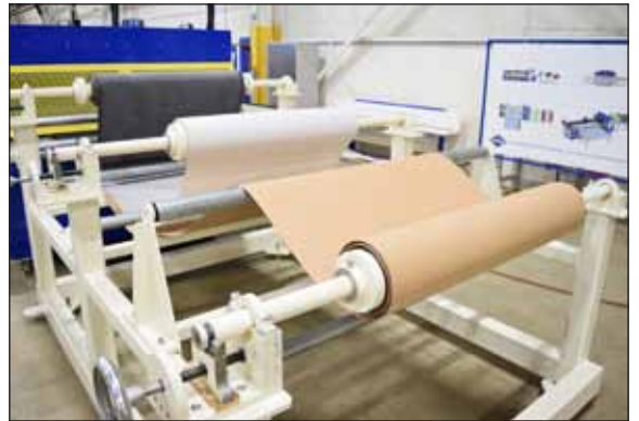
The roll handling system can fit up to three rolls of material to feed into the waterjet.
