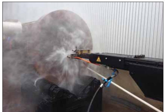
Inside Bundle Cleaner 5 (IBC-5) with optional rotating gun nozzles for hands-free cleaning of tube sheet.
