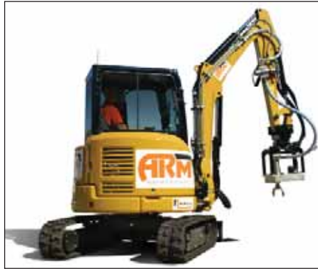
The ARM lets an operator control waterjets from the cab.
