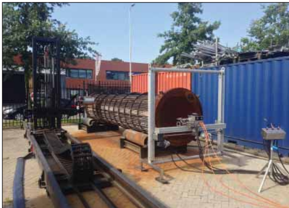
Outside Bundle Cleaner-C (OBC-C) and the standard indexing frame with 3XLTC used for cleaning bundles in the cleaning bay.
