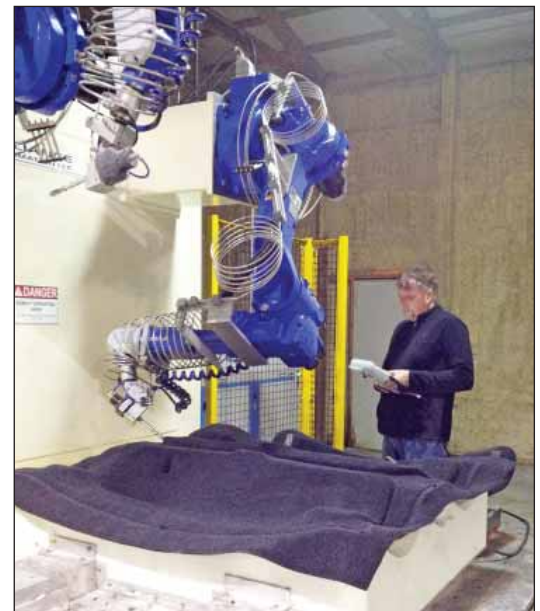
Alliance Automation's robotic waterjet trimming cell allows many different parts to be programmed so tools or products can be quickly changed. Programming is accomplished via the Teach Trace Method. Control/Program Engineer Photo credit: Alliance Automation, LLC
