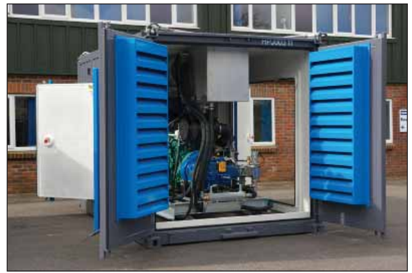
Twin doors on three sides for unrestricted access for maintenance.
