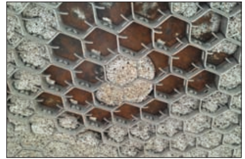
Figure 7. Partial Removal by 3-D Due to Mesh Shadow in AA-22 Refractory.
