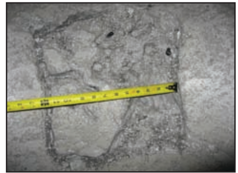
Figure 1. Results of Manual Chipping in Type 1 Refractory, 1 Hour Duration.
