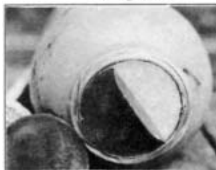
Russian water bomb (mine) filled with 32 kilograms of TNT cut to open top for TNT washouts.
