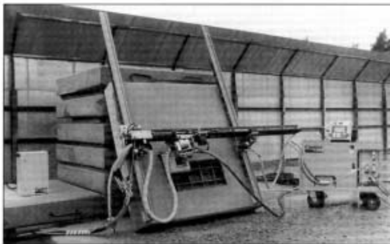
The new compact and lightweight Conjet Jetframe 102 system selectively removes damaged concrete in confined spaces and on surfaces inaccessible to standard Conjet hydrodemolition equipment.
