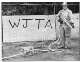
Jetech demonstrates the power of its jet gun by cutting the WJTA logo in 1/2" plywood.
