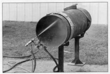
Jet Edge, Inc. demonstrates its abrasive jet pipe cutter.
