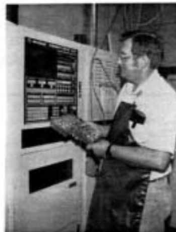
Computerized controller for PASER II™ abrasive jet cutting system
