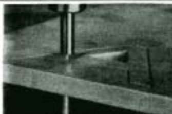
Abrasive water jet cutting the letter A from a piece of 1/2" thick aluminum Photo courtesy of Ingersoll-Rand Waterjet Cutting Systems, Baxter Springs, Kansas
