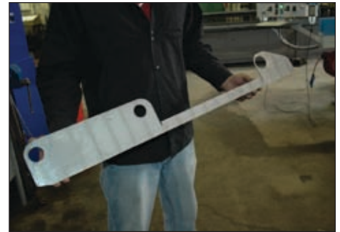
Baffle plate material 0.120-inch thick cut from 1/8-inch mild steel.
