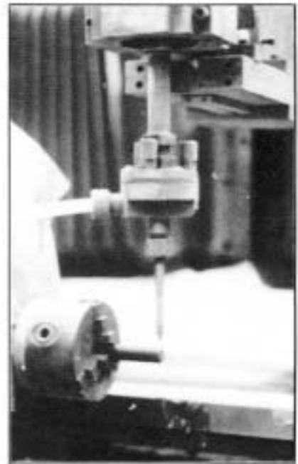
Screw thread machining of a composite rod.
