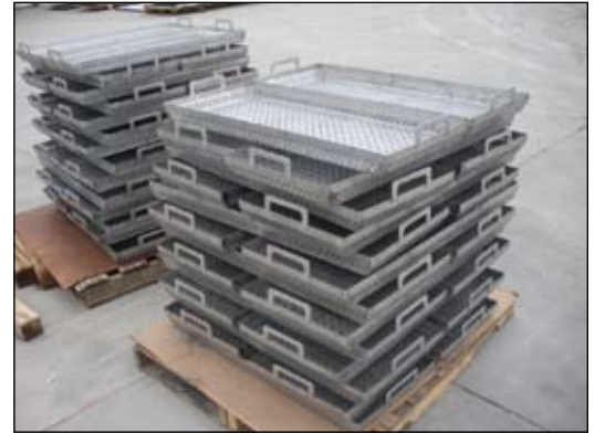
The basic stainless steel components of these industrial-sized vegetable and rice steam trays were cut from FusionTECH’s OMAX 80160 JetMachining Center.
