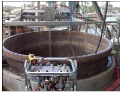
Transfer line exchanger mounted vertically with a "basic" remote control panel and high-performance pump controls.
