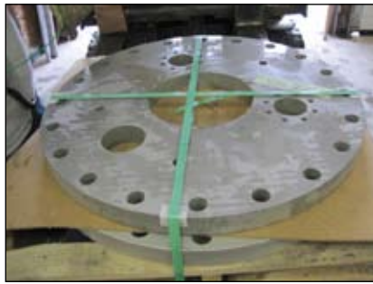
A 40-inch diameter ring flange was cut from a two-inch thick stainless steel slab by FusionTECH's OMAX waterjet equipment.
