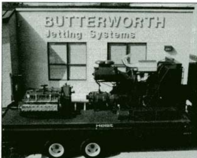
Butterworth's new 500 hp Liqua-Blaster unit offers pressures to 20,000 psi and flows to 153 gpm.
