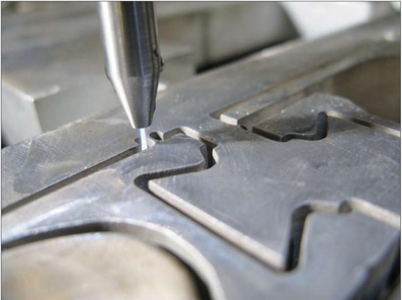
Waterjet maximizes material usage by cutting intricately nested parts out of 1 inch thick aluminium.
