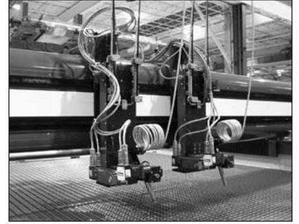
Many bridge designs are also built to be very light for waterjet cutting just like the cantilever counterparts, so simply going for a bridge design is not enough if you are looking to add other processes. For a machine to be able to add drills, tapping systems, height sensors, crash sensors, 5-axis cutting
