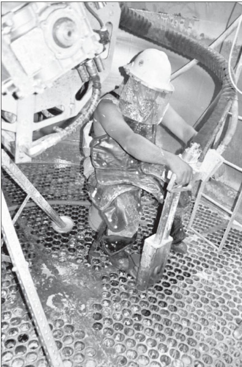
Operator inserts dual lance assembly powered by Jetstream UNx™ to hydroblast tubes.
