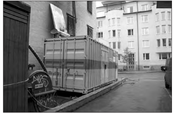
The Aquajet System's Ecosilence Power Pack not only meets noise levels of less than half that of conventional power packs, it also provides the contractor with significant fuel savings.
