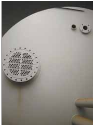
Inside horizontal confined space showing horizontal heat exchanger and flanged/unflanged lines.
