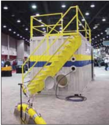
Rear of intermodal training simulator showing horizontal confined space entry, 4- and 6-inch line cleaning stations.
