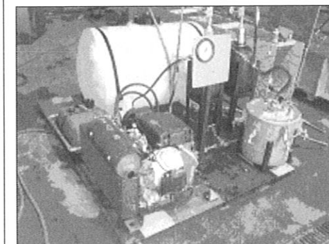
Figure 8. Pump and Slurry System
