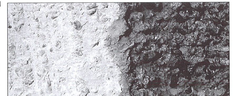
Rotomilled surface on left contains damage while the waterjetted surface on the right is fracture-free and has the roughness of gravel. Photograph courtesy of Dan Bernard, Resto-Tech Ultra Pressure Systems Ltd.
