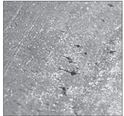
Figure 2. Detail of Corrosion Pits in Stainless Steel Tube
