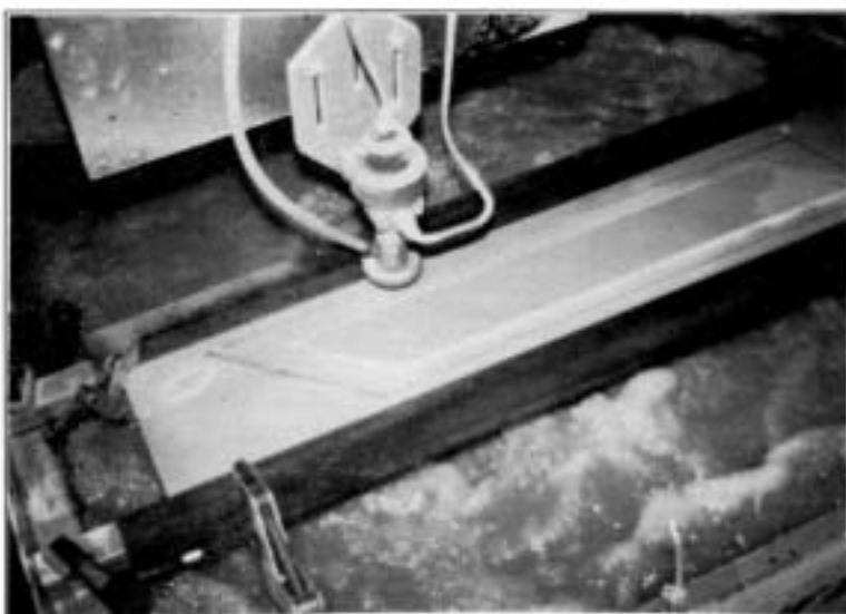
With the plate clamped onto the table, the last of the 9,290 holes are cut.
