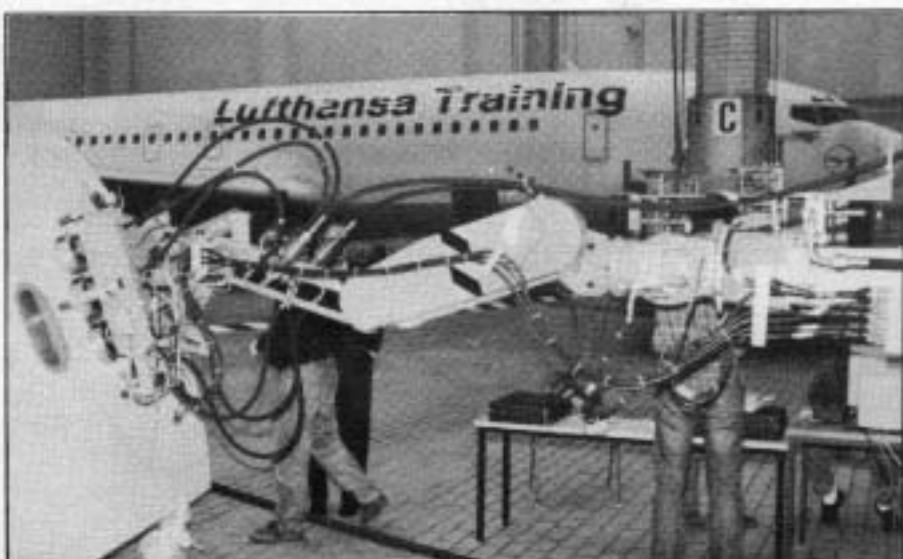
Stripping paint from an airplane. Photograph courtesy of WOMA Apparatebau GmbH, Duisburg.
